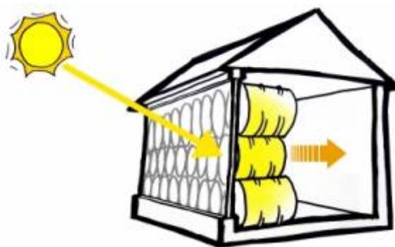
Figure 8: Barrels of water used as a heating material[5]
