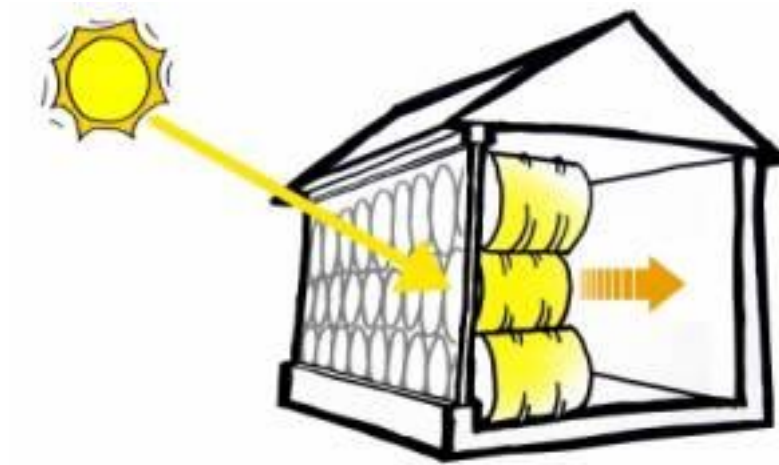
Figure 8: Barrels of water heat the greenhouse [5]
