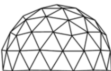
Figure 29: Geodesic dome made of triangles
