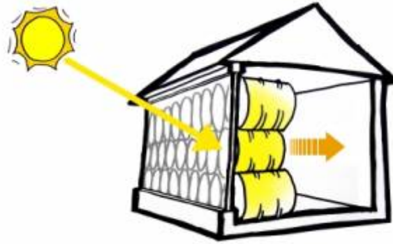
Figure 8: Barrels of water used as a heating material [5]
